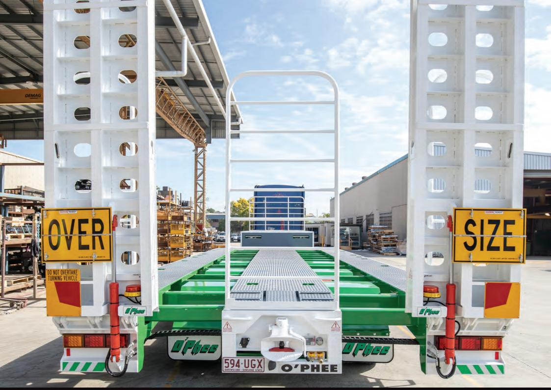
Unique heavy duty 'Widening' frame with ONE-PIECE Gooseneck web.
