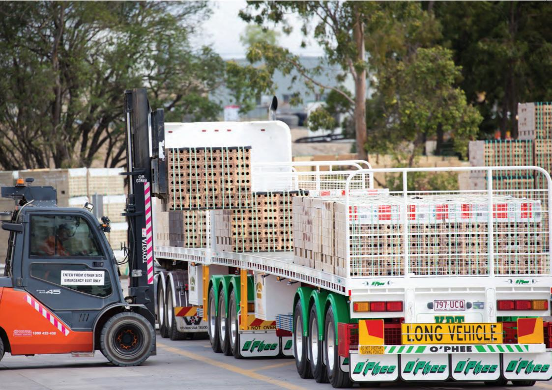
Unique frame design with matching beams. Coaming is 4" RSJ Hi-tensile with 1" tierail. Jost Landing legs, king pin & Turntable on Lead. Flooring 3mm checker plate. Storage - 1x lockable toolbox. DG (Flameproof) lighting. Stainless Steel Water Tank.
