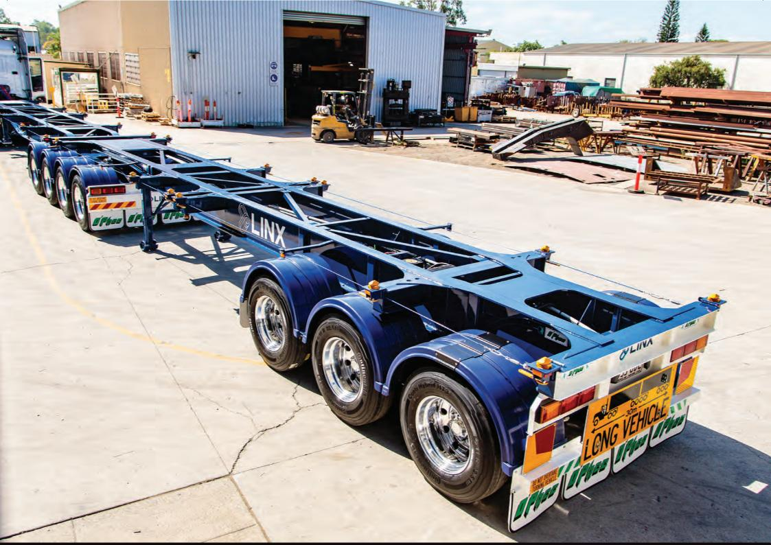
Unique frame design, matched beams. Lead 1x20' / Rear 1x20'-2x20'-1x40'. Jost Landing legs, king pin & Turntable (on Lead). Truckmate Plastic Guards.
